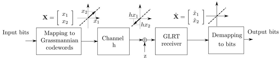
Fig. 2. Block diagram of a non-coherent transceiver with  $M = 1$  antenna and  $T = 2$  channel uses.
