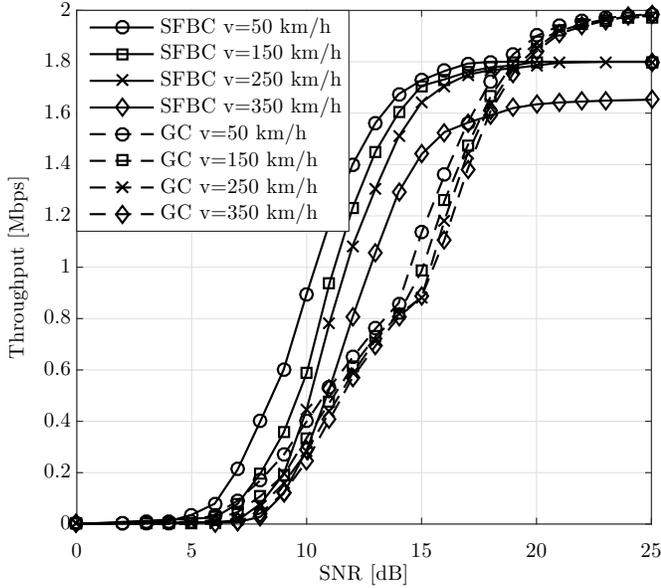
Fig. 3. Performance comparison among coherent and non-coherent schemes with uncorrelated antenna correlations in a  $2 \times 2$  setup.
