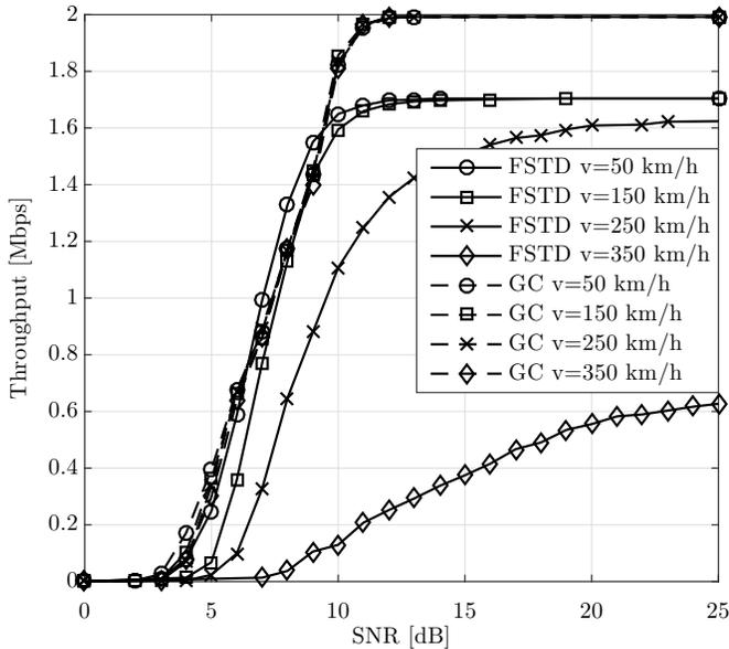
Fig. 4. Performance comparison among coherent and non-coherent schemes with uncorrelated antenna correlations in a  $4 \times 4$  setup.
