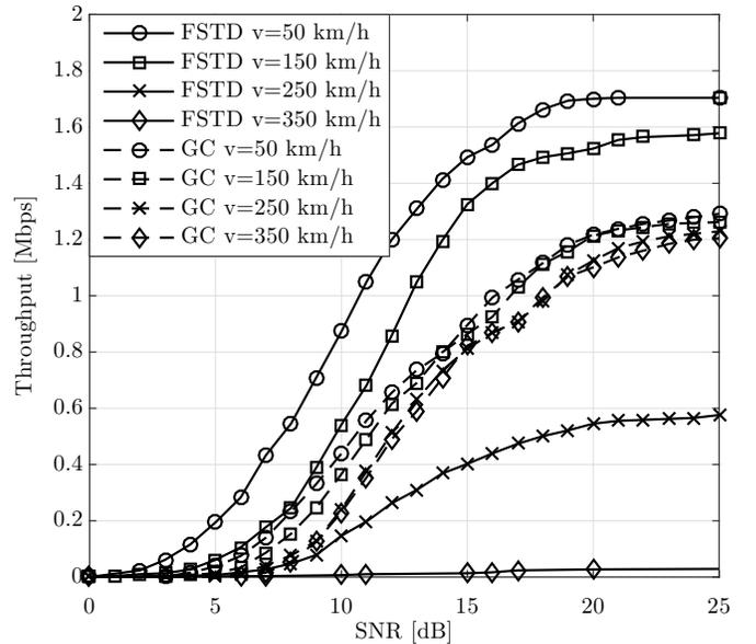
Fig. 6. Performance comparison among coherent and non-coherent schemes with high antenna correlations in a  $4 \times 4$  setup.
