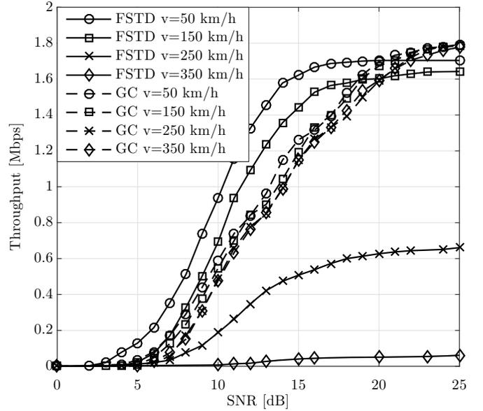
Fig. 5. Performance comparison among coherent and non-coherent schemes with medium antenna correlations in a  $4 \times 4$  setup.
